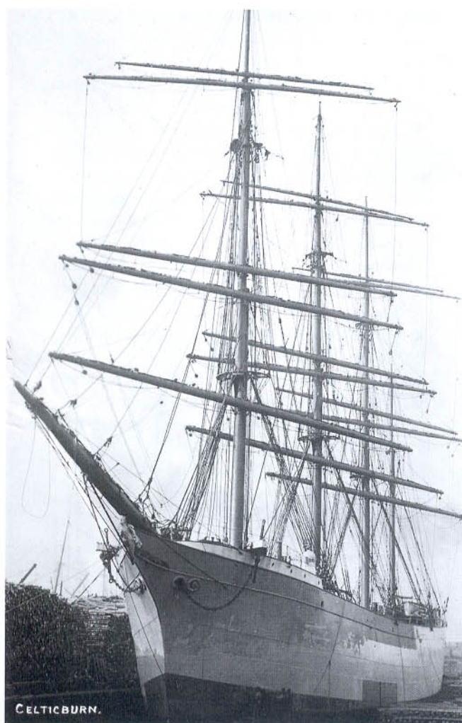
The heavily-rigged Celticburn was one of six baldheaders built by Barclay, Curle for Shankland's Burn Line. [John Naylor collection]
